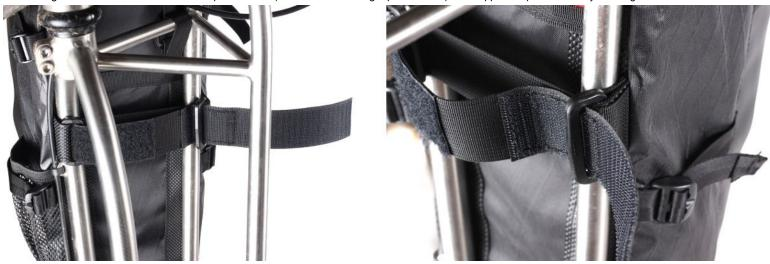
Step 5: Install the lower strap from front to rear over the front leg of the truss fork, through the D-Ring at the leg of the truss fork, and pull back toward front to tighten as shown in photo below.
