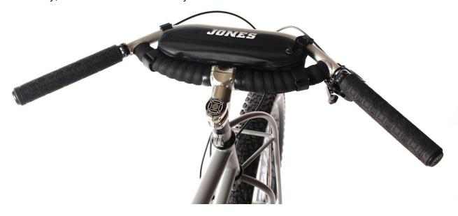
Warning: All four (4) main straps must be secured around the tubes of the H-Bar at all times to ensure your safety. Make sure to check that the four (4) main straps are secure before each ride because they are critical for the pack's stability. Check your H-Bar Pack and its attachment straps for damage with every ride. If the H-Bar Pack is not attached correctly or is damaged it can come loose and get caught in your wheel causing serious injury.
