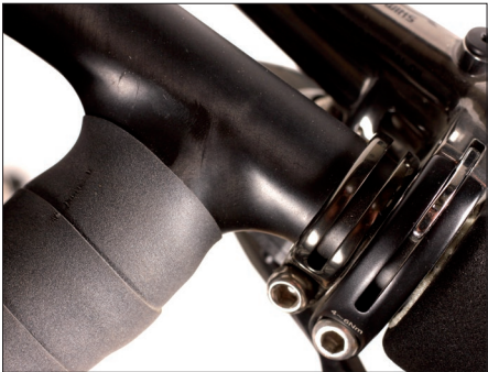
Above, correct lever position on carbon H-Bar™
