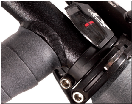
Above, correct lever position on aluminium H-Bar™
