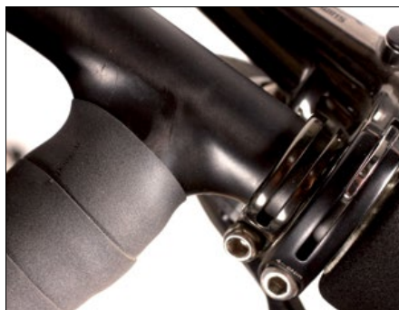
Above, correct lever position on carbon H-Bar®
