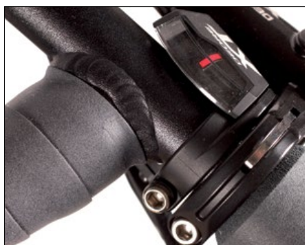
Above, correct lever position on aluminium H-Bar®
